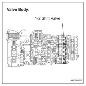
The 1-2 shift valve performs shifting to 1st gear and other gears.
